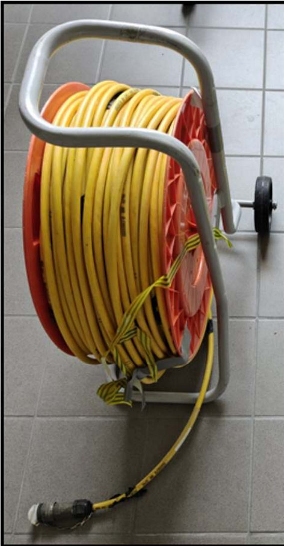
Traditional 24 ch 5m spacing cable 24 kg
